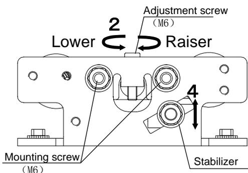
3. Tighten the mounting screw.
