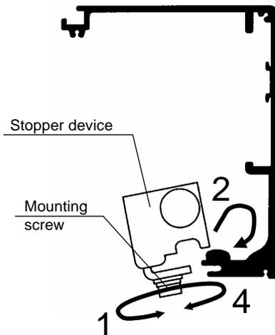
1. Loosen the mounting screw(M8×40).
