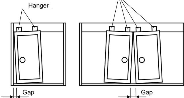
If the door can not be installed horizontally as shown left figure, it can be adjusted after it is hung on the Engine case.
