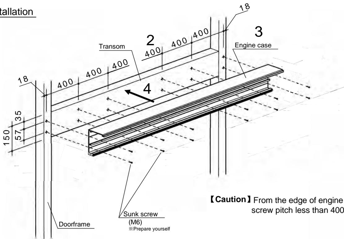
**【Caution】** From the edge of engine case, keep screw pitch less than 400mm.
