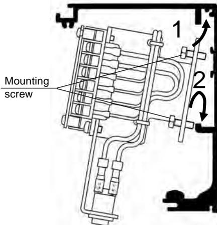
1. Insert the Terminal device into the upper groove.
