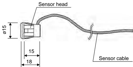
1. Drill holes in the frame so that the sensor heads can be mounted in a recessed position with the lenses directly facing each other.
