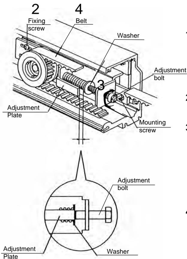
1. Pull the Jockey wheel device to the left side by hand to tighter the belt, then, keeping the belt taut, tighten the 4 mounting screws.
