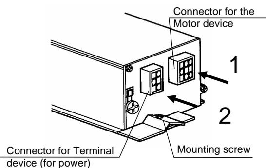
1. Connect the Motor device lead wire to the Control device.
