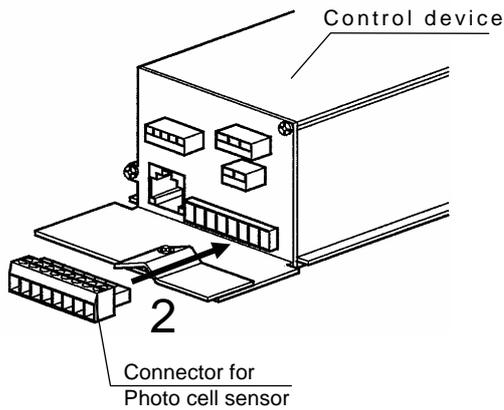
1. Peel the external cover of the Photo cell sensor cable, and connect it to the connector.
