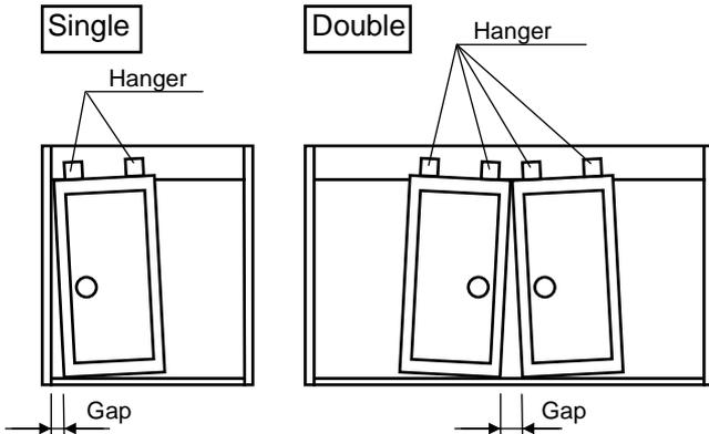
If the door can not be installed horizontally as shown left figure, it can be adjusted after it is hung on the Engine case.
