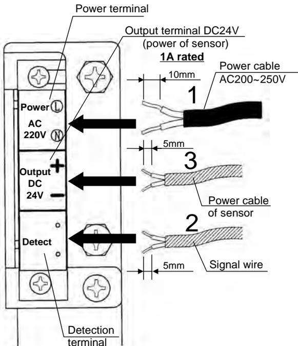
1. Connect the power cable to the power terminal securely.
