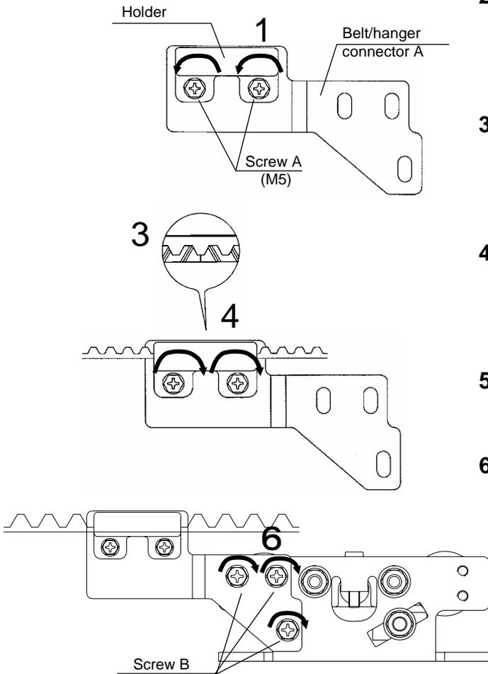
1. Loosen the screw A(M5) and remove the Holder from Belt/hanger connector A.
