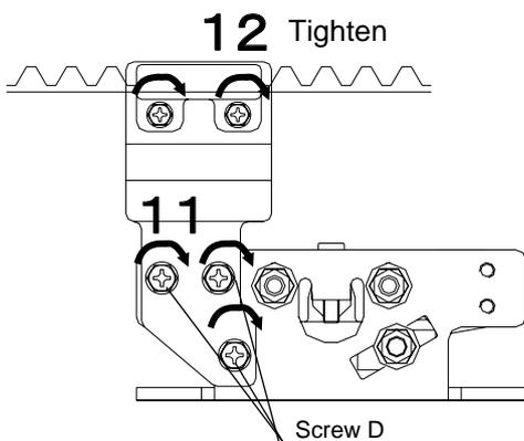
7. According to **18•Belt Tension Adjustment (P.26)**, adjust the belt tension.
