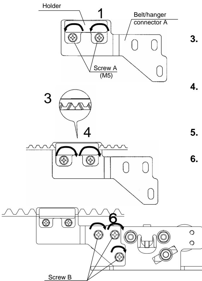
1. Loosen the screw A(M5) and remove the Holder from Belt/hanger connector A.
